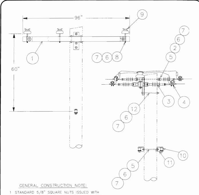
1 STANDARD 5/8" SQUARE NUTS ISSUED WITH DA BOLTS, MH BOLTS AND STEEL INSULATOR
