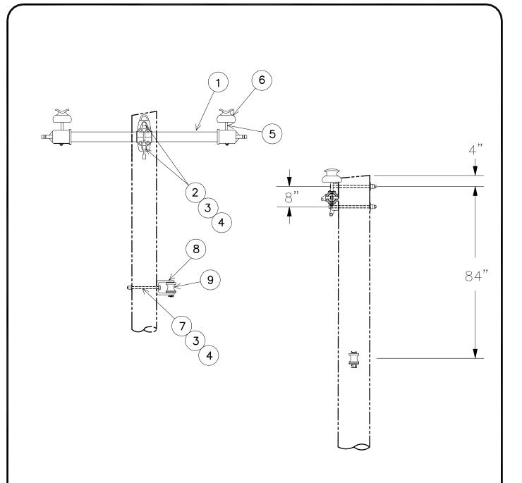
ENGINEERING NOTE: NEUTRAL MAY BE INSTALLED AT 60" TO MEET EXISTING FIELD CONDITIONS.
