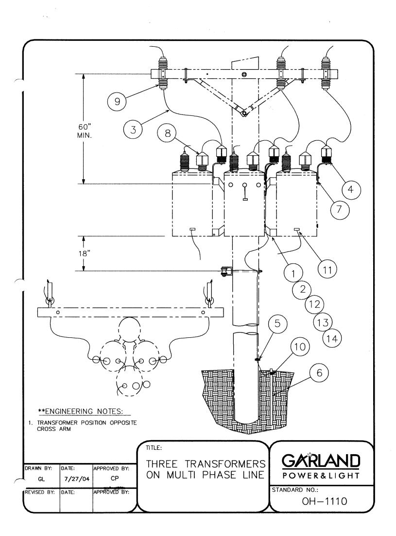
PRIMARY.-DELTA EACH TRANSFORMER IS ENERGIZED BY TWO PHASES FROM THE PRIMARY CIRCUIT. TWO BUSHING TRANSFORMERS RATED FOR 12470 ARE USED. THE SYSTEM GROUND IS ONLY USED FOR CASE GROUNDING AND SECONDARY GROUNDING. THE TRANSFORMERS MUST MATCH WITH REGARD TO IMPEDANCE. EXCESSIVE CIRCULATING CURRENTS MAY OVERHEAT AND BURN OUT THE TRANSFORMERS IF THEY ARE NOT THE SAME.
